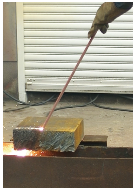
5. 厚鋼板(120mm)の熔断
