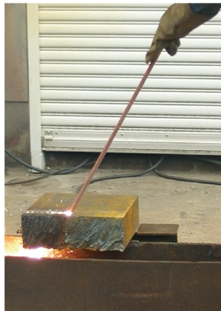
5. 厚鋼板(120mm)の熔断
